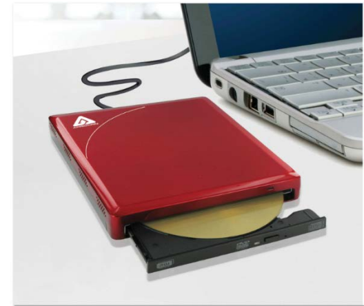
FIGURE 3-12 External optical drives. Can be connected as needed, typically via a USB port, such as to the netbook shown here.
