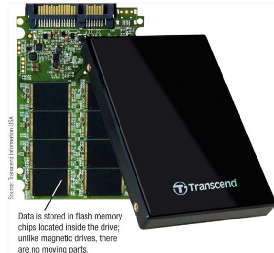
FIGURE 3-7 Solid-state drives (SSDs). Contain only flash memory.
